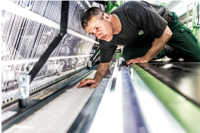
Figure 5: Production of a cured-in-place pipe preproduct in the factory (Source: SAERTEX multiCom GmbH)
