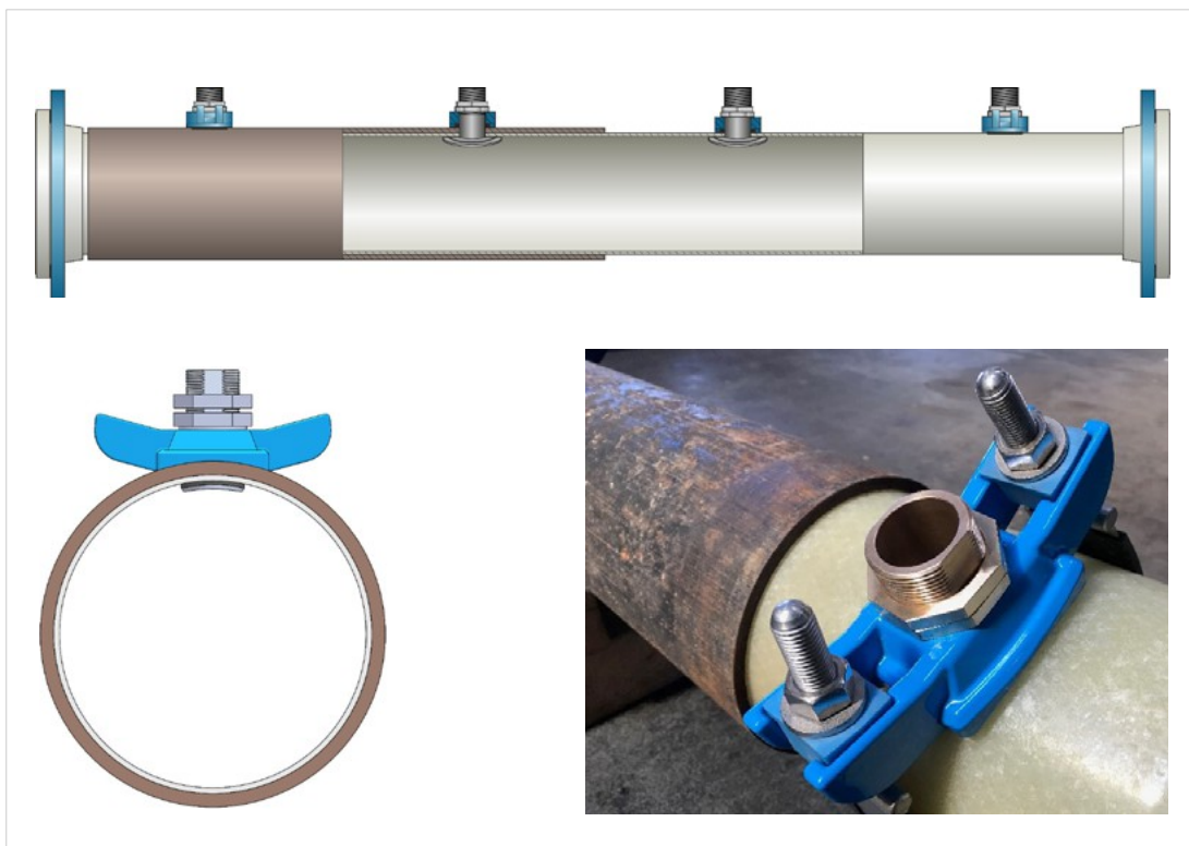
Figure 6: Connection fitting with internal seal consisting of an internal and external saddle - on the renovated pipe (left) or directly on the liner (right)
